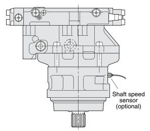
V14-160 (AC control) with speed sensor.
