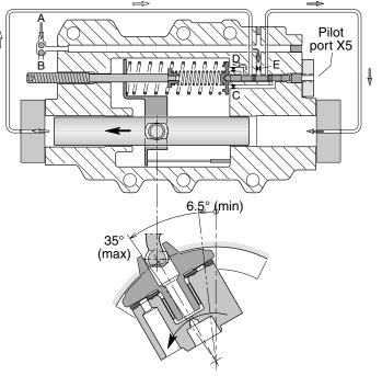
EP control function (displ. decrease at increasing current). HP control function (displ. increase at decreasing pilot press.).
