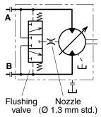
Hydraulic schematic - V14 with built-in flushing valve.
