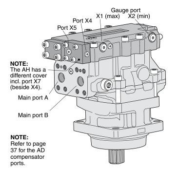
Port locations - V14- with AC or AH compensator.
