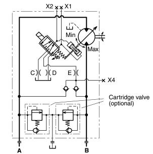
EP schematic (shown: non-activated solenoid; control moving towards max displacement).
