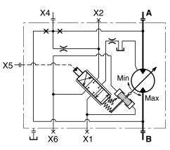
HP S 01 E schematic (spool in a balanced, mid-pos.).
