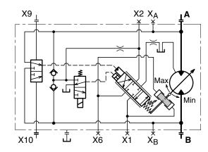
AE schematic (spool in balanced, mid-position).
