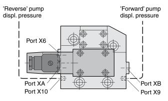
AE end cover with solenoid valve and brake defeat.
