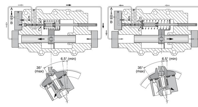
AC function (displ. increases at increasing system pressure). AC function (displ. decreases at decreasing system pressure).
