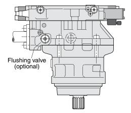
V14-110 (EP control) with built-in flushing valve.
