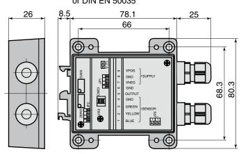
Electronic module (incl. internal programming module).
