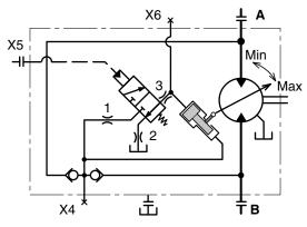
T12 schematic (no pilot pressure; the control is in max displacement position).
