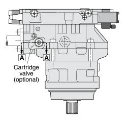
V14- 110 (EP control) with relief valve cartridges.
