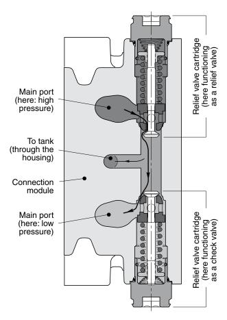
Section A-A (showing pressure relief cartridges).
