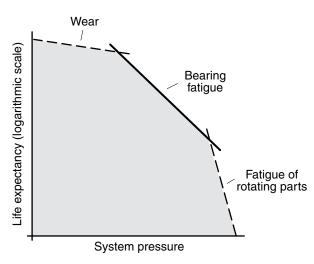
Hydraulic motor life versus system pressure.
