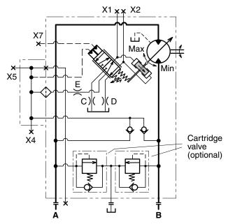
AH schematic (shown: override port X7 not pressurized; the compensator is moving towards min displacement).
