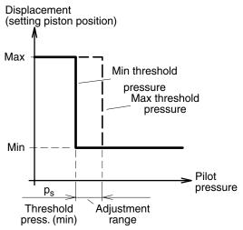
HO diagram (displacement vs. pilot pressure).
