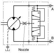
T12 with flushing valve block type FV.
