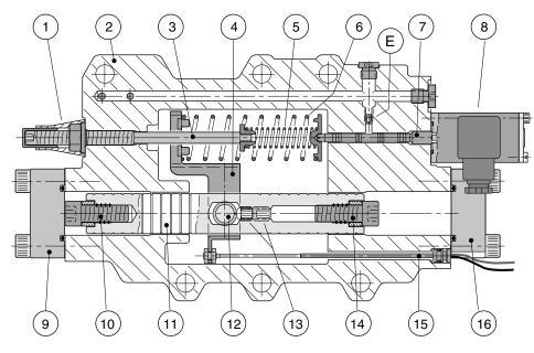
Cross section of the EP control module.
