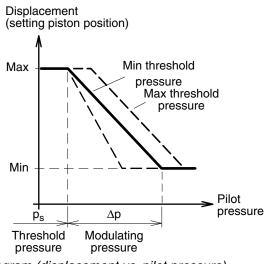
HP diagram (displacement vs. pilot pressure).
