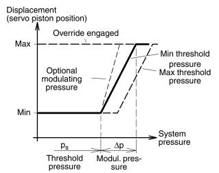
AH diagram (displacement vs. system pressure).
